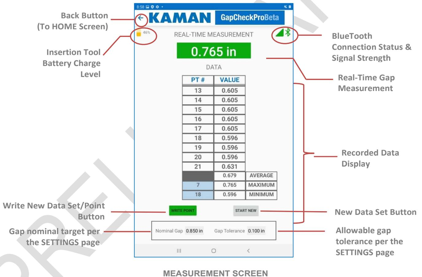
The screenshot shows the 'MEASUREMENT SCREEN' of the KAMAN GapCheckProBeta application. The screen displays a real-time gap measurement of 0.765 in in a green box. Below this is a table of recorded data points. At the bottom, there are buttons for 'WRITE POINT' and 'START NEW', and a section for 'Nominal Gap' (0.850 in) and 'Gap Tolerance' (0.100 in). A Bluetooth connection status icon is visible in the top right corner.
