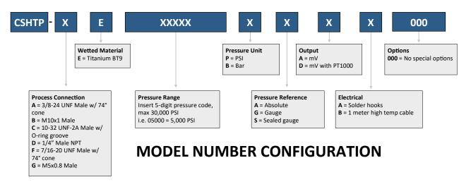
Ordering Example: CSHTP-AE01000BSAA000 (3/8-24 UNF Male w/ 74° cone, Titanium BT9, 0-1000 Bar sealed gauge, mV, Solder hooks) Not all configurations are available. Our sales team can recommend the closest available configuration based on your requirements. Contact Core Sensors for configurations not shown. Visit our <u>How To Buy</u> page or <u>contact us</u> for a quote.
