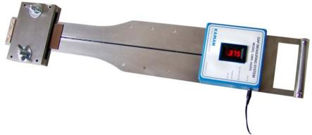
While pushing down on the .375" Calibration Plate, tighten the wing nuts until the Calibration plate is firmly seated on the Base Plate. Check to make sure both of the legs on the Calibration Plate are in full contact with the Base Plate.
