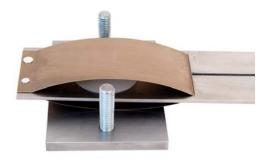
Place the .250" Calibration Plate over the upper spring with guide pins aligned in the holes. Install a washer and wing nut on each guide pin.
