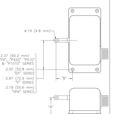
\* With "DS" (dust shield) option, add 0.36" (9.1 mm) to "B" dimensions above.
