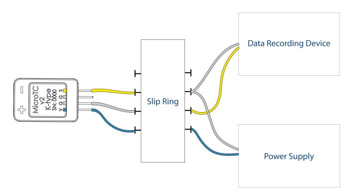
The thermocouple sensor should be attached using the provided mating connector (Omega± HMPW-\*-M). If a thermocouple input is left unused or if the thermocouple opens, the output of the amplifier will rise to V+. The amplifier will not be damaged if a thermocouple is left unattached.
