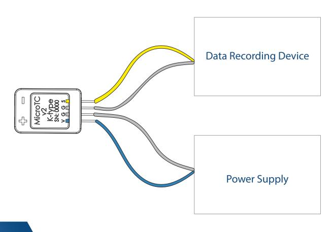
The output high is measured relative to the ground wire. It is recommended that a separate wire for signal common is added to the common terminal to reduce errors from voltage drops along the power common wire. When using the MicroTC with a slip ring assembly, a separate signal common can be added to the stator of a slip ring to decrease the amount of rings needed, but it is important to place the amplifier as close as possible to the slip ring.
