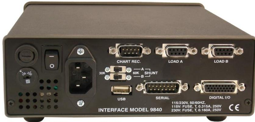
Next connect a load or torque cell to the 9 pin female connector labeled “Load A”. You should use the cabling supplied with your Model 9840 and Interface load or torque cell. If you do not have a factory supplied cable see Appendix B for the recommended cell connection.
