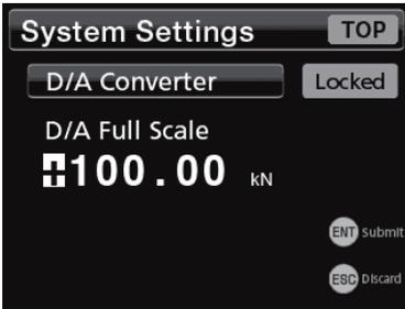
The following is an example of when "9-2-4. D/A Max. Voltage" is set to 10V.
