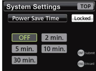
To change a setting value when locked, from the Function Menu, select System Settings → Lock, and disable locking for the calibration or setting values (page 35).
