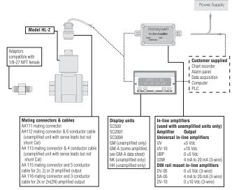
NOTE: For long cable runs or electronically noisy environments, an amplified sensor or locally mounted amplifier is often preferred.
