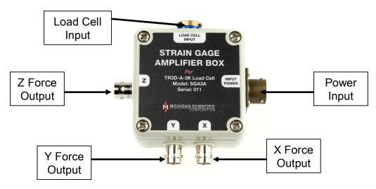
2. Connect the  $\pm 15$  VDC power source to the Amplifier box using the Power Input connector. The pin out for this connector is in the table below. A mating connector and cable is provided.
