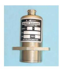
The Jewell ASXC Series Fluid Rotor Angular Accelerometer is a force balance servo accelerometer that uses a fluid-filled ring chamber to measure angular acceleration. The ASXC is currently used in a wide variety of applications including many military and aviation flight controls including autopilot or aircraft stability and control systems or satellite stability.
