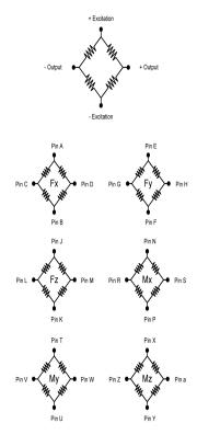
Bridges Fz; Mz = 700 ohms Bridges Fx; Fy; Mx; My; = 350 ohms Connector Type: Souriau 851-02E16-26P50-44
