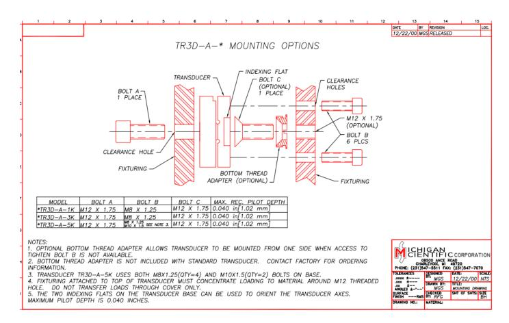
In cases where access is not available to mount the Load Cell base with four bolts, an optional Bottom Thread Adapter should be used. This Adapter threads into the base of the Load Cell and "captures" a flat-head socket cap screw. The tightening "key" for this screw is accessed through the top mounting hole of the Load Cell.
