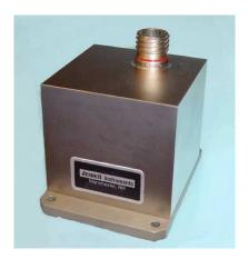
The Jewell LCF-2310 Series is an extremely rugged biaxial fluid damped flexure suspension servo Inclinometer designed for industrial, commercial and aerospace sensing requirements. The seal of the LCF-2310 is splash proof making it ideal for outdoor use.
