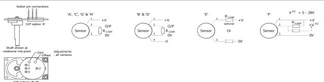
**Gain and Offset Adjustment:** (Typically  $\pm$  10% Min available) To adjust the gain or offset use a small potentiometer adjuster or screwdriver 2mm across. Do not apply too much force on the potentiometers. The offset is set at mid span at the mid point, within  $\pm$ 5°, of rotation.
