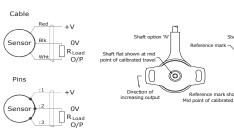
**Mechanical Mounting:** Flange mounted. The flange slots are 4.5mm by 20 degrees wide, 48mm pitch. The sensor should be mounted with minimal axial and radial loading on the shaft for optimum life. It is recommended that the shaft is coupled to the drive using a flexible coupling. Option 'N' shaft:  $\emptyset$  4 mm x 8 mm long, flat 3 mm A/F x 4 mm. Option 'P' shaft: fits 6 x 3 mm slot.
