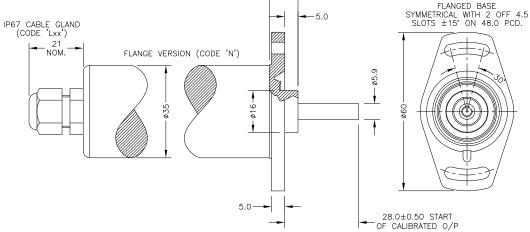
IP67 SHORT CABLE GLAND (CODE 'Mxx') NOTE: SENSORS ARE MADE IN FOUR STANDARD LENGTHS. --- 2 NOM. TRAVEL: (mm) BODY LENGTH: (mm) CALIBRATED MECHANICAL 'X' STANDARD Y' FLANGE 0-51 TO 0-70 70 0-71 TO 0-100 100 141.3 171.3
