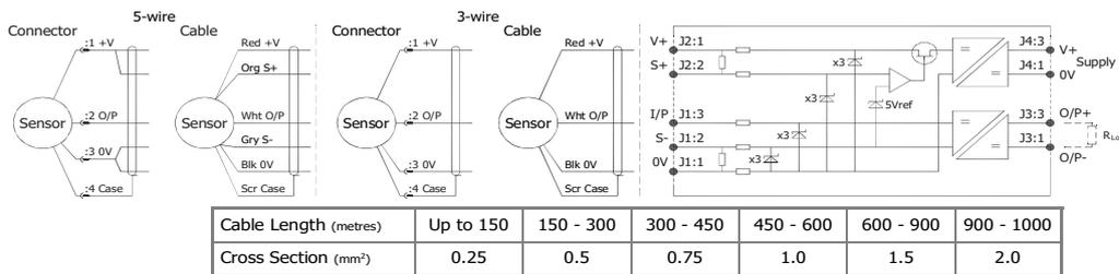
The table above shows recommended conductor sizes with respect to cable length for both three and five wire connections, based on copper conductors. Three wire connections will introduce a gain reduction of 5% and a ±1% temperature dependence of gain over the range -40°C to +80°C for the cable temperature. (i.e. about -150 ppm/°C for the maximum lengths shown and less pro rata for shorter lengths.)
