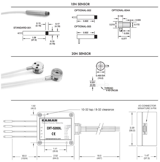
*Note: All dimensions shown in inches (mm). Standard enclosure. Note: Single channel systems use the x axis sensor connectors.*
