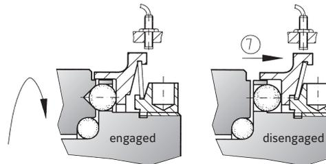
With this design, when a torque overload is detected, the disc spring completely flips over and places no residual spring pressure on the actuation ring. The drive and driven elements are completely separated.
