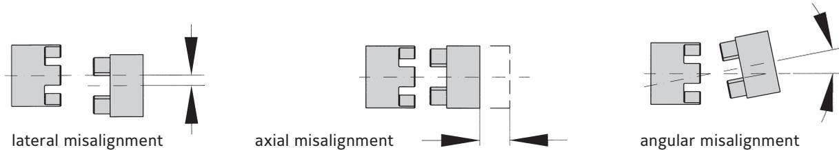
**!** In Table 2 you will find the maximum permissible values for the three axis of misalignment. It is important to remain within these limits to ensure long life and proper operation of the coupling. If several misalignment types occur at the same time, it is necessary to reduce the maximum permissible misalignment values. The percentage of the maximum value summing up actual misalignments must not exceed 100 %.
