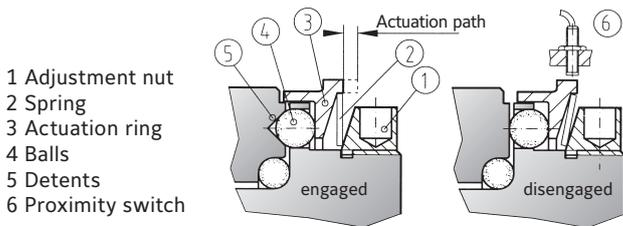
In a torque overload, with the single-position design (standard) and multi-position design, the spring disengages to allow the balls to come out of their detents, separating the drive and driven elements. Very low residual spring pressure remains so that the coupling will re-engage once the torque is reduced below the overload setting.)
