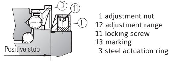
At ES 2 couplings, the slot of the clamping hub serves as a marking (13).
