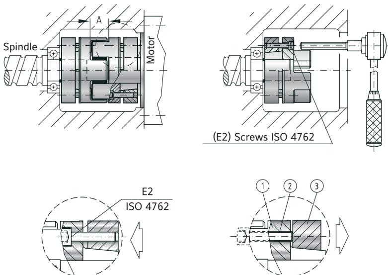
The EK6 uses a clamping ring with axial fastening screws (E). Slide the coupling hub onto the first shaft. Using a torque wrench, tighten bolts uniformly in circular sequence (not in a star pattern) to 1/3 of installation torque value. Next, tighten each bolt to 2/3 installation torque value in same manner.
