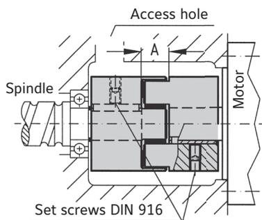
Slide a coupling half onto the shaft to the correct axial position. Tighten the set screw(s) to the appropriate torque using a torque wrench. Insert the elastomer ring and press the two coupling halves together. Make sure that the fit length (A) is maintained (see table 2). Mount the assembled coupling onto the second shaft and tighten the set screw(s).
