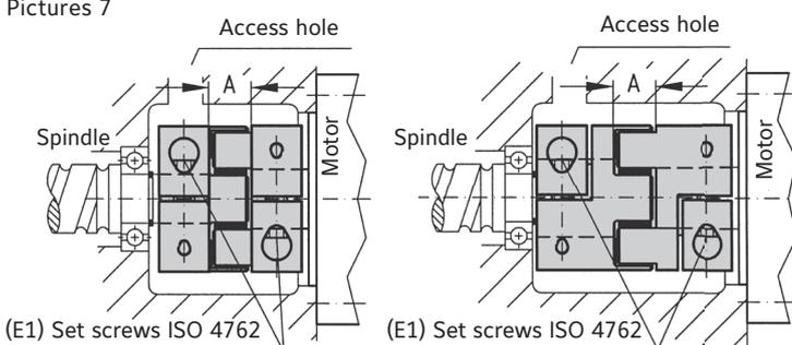
Slide a coupling half onto the shaft to the correct axial position. Using a torque wrench, tighten the clamp screw (E) to the appropriate torque indicated in Table 2. Insert the elastomer ring and press the two coupling halves together. Ensure that the fit length (A) is maintained (see table 2). Mount the assembled coupling onto the second shaft and tighten the clamp screw (E).
