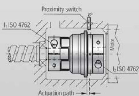
**Mounting:** Slide the coupling on the shaft ends to the proper axial position. Using a torque wrench, tighten the clamp screws to the correct tightening torque as indicated.
