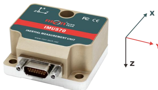
Fig. 1 Space coordinate system of micro-gyroscopes
