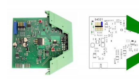
The input sensitivity can be adjusted by moving the jumper. The input sensitivity for position 1 is indicated in the type designation. In position 5, the amplification can be set in a continuously variable manner using trimmer "TR".
