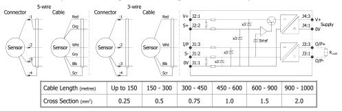
The table above shows recommended conductor sizes with respect to cable length for both three and five wire connections, based on copper conductors. Three wire connections will introduce a gain reduction of 5% and a  $\pm 1\%$  temperature dependence of gain over the range -40°C to +80°C for the cable temperature. (i.e. about -150 ppm/°C for the maximum lengths shown and less pro rata for shorter lengths.)
