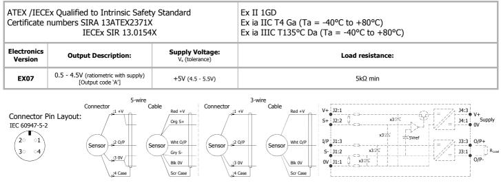
**Putting Into Service:** The sensor must be used with a galvanic isolation barrier designed to supply the sensor with a nominal 5V and to transmit the sensor output to a safe area. The barrier parameters must not exceed:-
