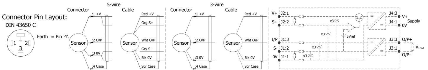
**Putting Into Service:** The sensor must be used with a galvanic isolation barrier designed to supply the sensor with a nominal 5V and to transmit the sensor output to a safe area. The barrier parameters must not exceed:-
