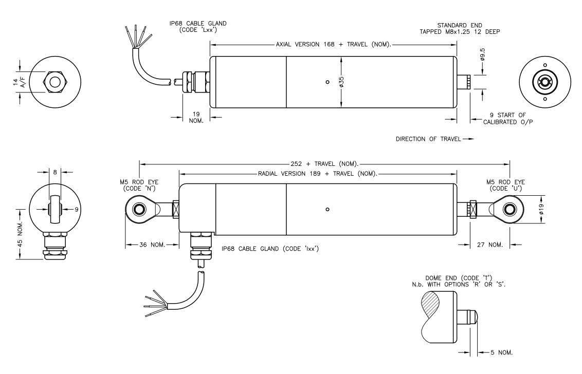
MAXIMUM WORKING DEPTH: 100 METRES/328 FEET. WHERE THE FREE END OF THE CABLE IS TO BE TERMINATED IN A SUBMERGED POSITION, ADEQUATE SEALING MUST BE PROVIDED TO PROTECT CONNECTIONS.
