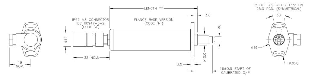
NOTE: SENSORS WITH TRAVEL UP TO 50mm ARE MADE IN STANDARD LENGTHS.
