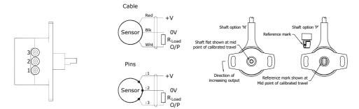
**Mechanical Mounting:** Flange mounted. The flange slots are 4.5mm by 20 degrees wide, 48mm pitch. The sensor should be mounted with minimal axial and radial loading on the shaft for optimum life. It is recommended that the shaft is coupled to the drive using a flexible coupling.
