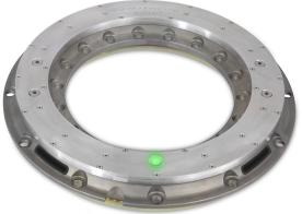
The *LW12.8-TEL Wheel Force Transducer (WFT)* is capable of measuring all of the wheel forces and moments on passenger cars and light duty trucks. It provides independent output signals for vertical, lateral, and longitudinal forces as well as camber, steer, and torque moments. It is completely weatherproof making it ideal for testing in any weather conditions.
