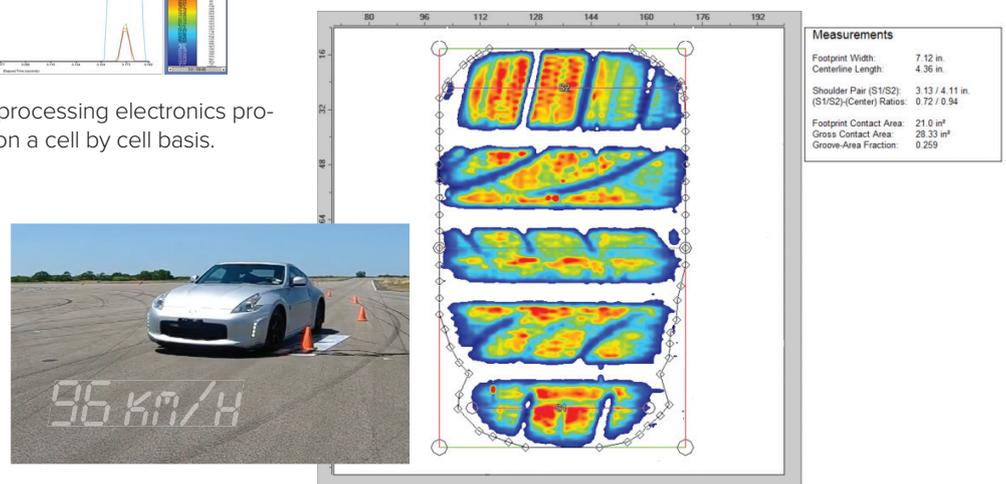
With 65,536 sensing points sampled at 450 fps, the HS Tire System generates high resolution images and accurate tire interface pressure data at speeds up to 140 km/h.
