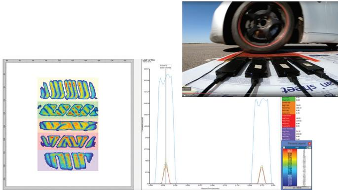
The HX510 sensor and ultra fast signal processing electronics provide consistent and repeatable results on a cell by cell basis.
