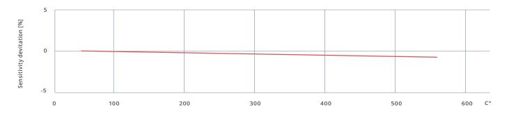
ISO 9001 certified calibration at  $+20^{\circ}$ C with dead weight tester (3, 6, 8, 10, 12, 20, 30, 50 bar). Sensitivity and linearity are determined according to DIN16086
