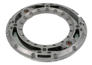
The *LW12.8-60 Wheel Force Transducer (WFT)* is capable of measuring all of the wheel forces and moments on passenger cars and light duty trucks. It provides independent output signals for vertical, lateral, and longitudinal forces as well as camber, steer, and torque moments. Being completely weatherproof, it is ideal for on-road and off-road measurements in all conditions. It can also be used to monitor and control laboratory tests.
