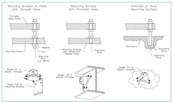
The drawing to the left illustrates installation techniques for 700-Series Biaxial Tiltmeters (Models 711-2, 716-2, and 712).
