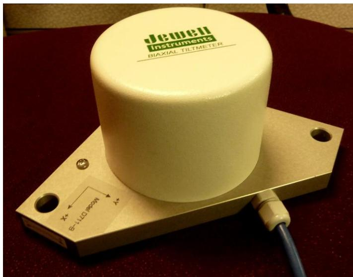
**Figure 1: Model D711 Digital Floor Mount Tiltmeter (Biaxial)**
