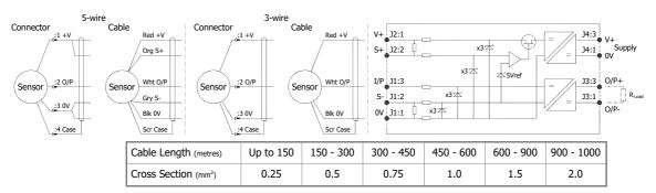
The table above shows recommended conductor sizes with respect to cable length for both three and five wire connections, based on copper conductors. Three wire connections will introduce a gain reduction of 5% and a  $\pm 1\%$  temperature dependence of gain over the range -40°C to +80°C for the cable temperature. (i.e. about -150 ppm/°C for the maximum lengths shown and less pro rata for shorter lengths.)
