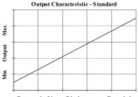
Retracted Linear Displacement Extended
