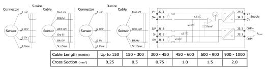
The table above shows recommended conductor sizes with respect to cable length for both three and five wire connections, based on copper conductors. Three wire connections will introduce a gain reduction of 5% and a  $\pm 1\%$  temperature dependence of gain over the range -40°C to +80°C for the cable temperature. (i.e. about -150 ppm/°C for the maximum lengths shown and less pro rata for shorter lengths.)
