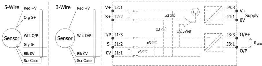
**Putting Into Service:** The sensor must be used with a galvanic isolation barrier designed to supply the sensor with a nominal 5V and to transmit the sensor output to a safe area. The barrier parameters must not exceed:-
