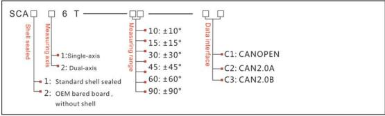
E.g: SCA126T-10-C1: dual-axis /standard/±10°Measuring range /CANOPEN output
