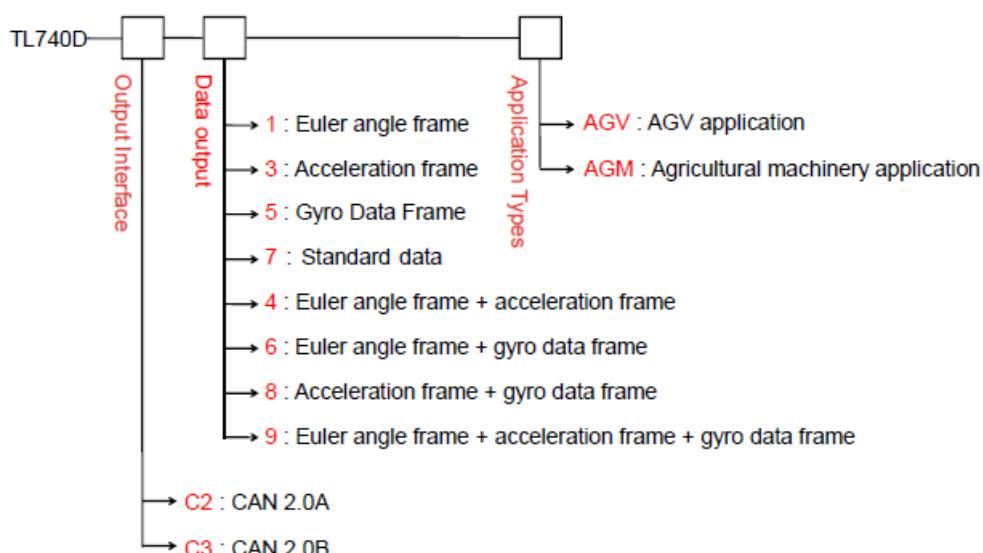
E.g : TL740D-C2-1-AGV : CAN2.0A Output Interface/Euler angle frame data output/AGV application.
