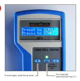
The LCT-Ultimate can also continuously display the **load cell signal in percentage** of L/C full capacity.
