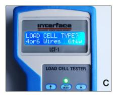
In order to save battery, the backlit LCD display turns off if nothing is done for 15 seconds. To turn the display on, just push any arrow key that won't affect your settings or your current menu. To shut off the unit, press the Enter key  $(\leftarrow)$  for a few seconds, or leave it on. It will turn off automatically after a few minutes.
