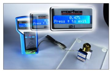
Apply 300g onto 45.4kg L/C, calculating the reading to be 0.91%
