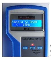
Note: LED turns red in case of low insulation resistance
