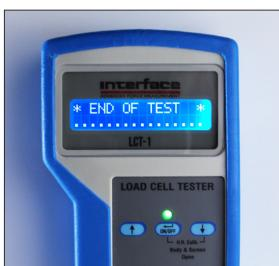
The unit will display "END OF TEST" when complete
