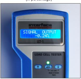
Note: When Load Cell is not loaded, the output should be around 0% (zero balance). Reference the loadcell specification for acceptable zero balance range.
