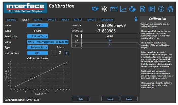
Polynomial calibration allows linearization of up to 11 points. Note that you must use the Points [+] button to add one point at a time. Once the polynomial value has been entered the button will be enabled to allow another point to be added.
