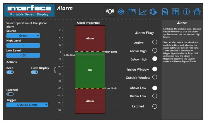
The single, global alarm acts on the currently selected calibration range (or TEDS device) and is solely based on the Source selected here.
