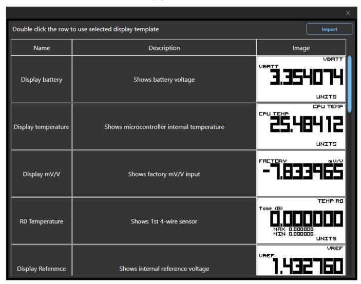
Here you can configure the user interface of the handheld and change settings of the backlight as well as the keypad.
