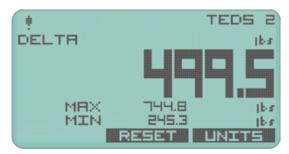
Soft keys allow the min and max to be Reset to the current value. i.e. zero the Delta. The usual Units selection is also available.
