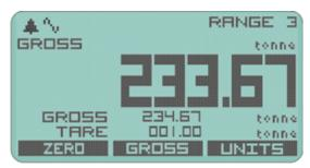
The Gross value and value of Tare are continuously displayed under the main value. Soft keys allow you to Zero the main display, switch back to full Gross value or change displayed units.
