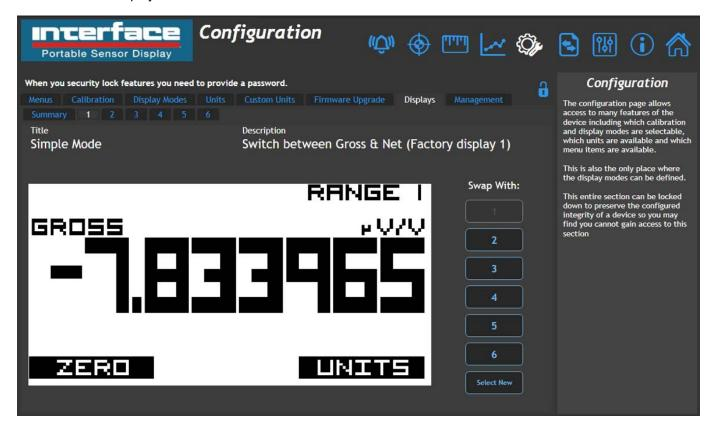
Configure the available Display Mode slots with the required Display Modes.
