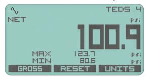
Soft keys allow you to toggle between Zeroed and Gross values as well as Reset the min and max to the current value. Units selection is also available.
