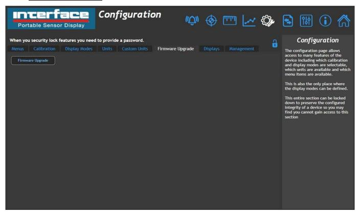
This section allows the firmware in the handheld to be updated.
