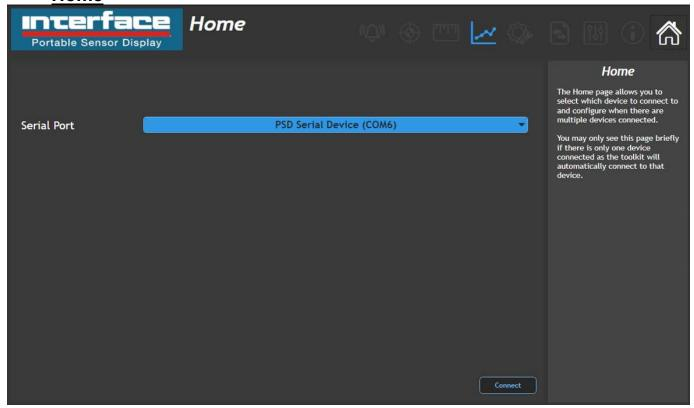
When you connect the handheld to the PC using a USB cable it creates a virtual COM port on the PC. All detected 9325 devices are displayed in the drop-down list, all you need to do is select the appropriate one. If only one handheld is detected, you may not see this page as the 9325 Toolkit will automatically select and connect to it.
