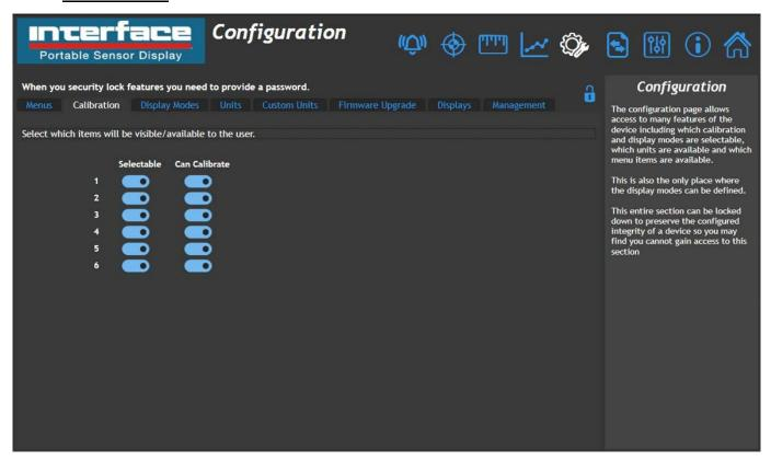
This section allows you to configure the available six calibration ranges availability from the menu and whether the range is selectable via the keypad (If that keypad action has been enabled).
