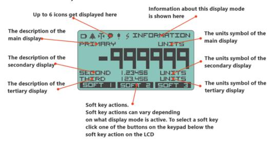
The values for the main, secondary and tertiary items are not indicated on the above diagram to improve clarity. Other modes such as the menu or editing values will be shown in the appropriate sections of the manual.
