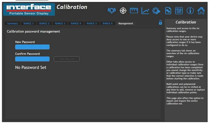
Allows setting a new password or removing an existing password to protect or release the calibration settings.
