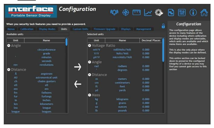
This section allows you to define which units of measure are available for calibration as the base engineering units and also any unit conversions that are selectable from the "Units" soft key that appears on most display modes. Two lists are displayed. The left one shows all available units that are not currently enabled and the one on the right shows the units that are available for calibrating or conversion.
