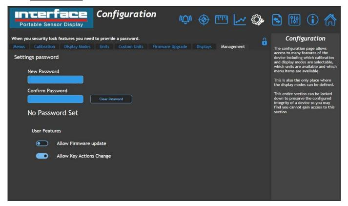
Access to the entire set of Configuration settings can be locked with a password. Without the password a user cannot change any of the protected settings which include the available Display Modes. This tab allows setting a new password or removing an existing password to protect or release the configuration settings.
