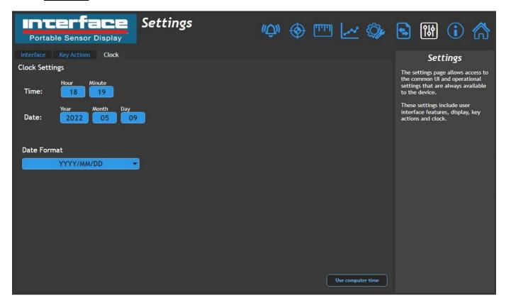
Here you can configure the device real-time clock.
