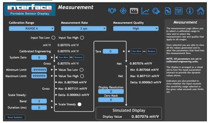
This page allows you to change the measurement settings. It is also presented in a way to visually represent how the parameters interact to generate the various dynamic result values. Each calibration range has its own set of these parameters and they will be remembered the next time the calibration range is selected.
