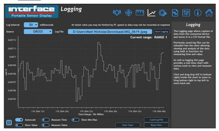
This page allows data from the handheld to be logged to a file and later reloaded to be viewed on the chart. A real-time chart is always visible whether logging is active or not.
