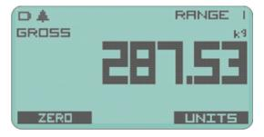
The current calibration range is displayed top right and Gross or Net is displayed above the main value. Current units are displayed above right of the main value.
