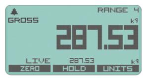
The other soft keys allow for the ability to Zero the main display or go back to displaying Gross. As usual, there is a soft key to allow for Units to be selected.
