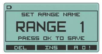
The text at the top inside of the box states what parameter is currently being edited. One of the characters will be the current selection and this character will flash alternatively displaying its character and an underlined space.
