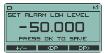
The text at the top right states the engineering units of the value being entered. The text at the top inside the box states what parameter is currently being edited. One of the digits will be the current selection and this digit will flash alternatively displaying its character and an underlined space.
