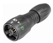
To attach this connector to the handheld, align the white arrow on the connector with the white line on the handheld socket. Rotate the locking collar as indicated on the connector. The connector fitted to the 9325 Standard Product is BINDER 770-8. The cable fitted mating connector is a BINDER 771 8-way male connector. This male connector is available under three different BINDER Order Codes determined by the field cable diameter.
