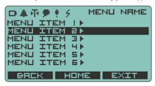
The currently selected menu item is displayed on a dark background and this selection can be changed by using the up and down keys. Pressing OK will select that item and can either:
