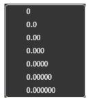
**Note:** The decimal places can also be modified (globally for the currently displayed engineering units) by using a long press on the keypad left and right direction keys (If this action has been allowed).
