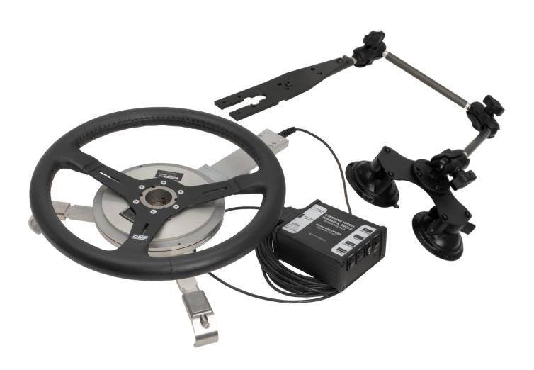
There are two optional mounting arrangements available. In both cases the user will interact with an aftermarket steering wheel which is bolted to the top of the transducer.
