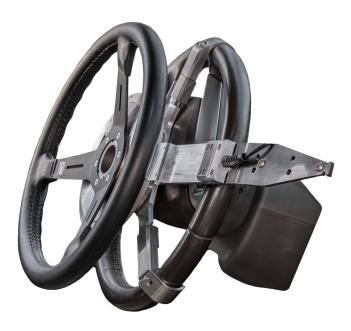
With the second option, the OEM steering wheel is removed, and the bottom side of the transducer is bolted to a custom spline adapter which mounts directly to the steering wheel shaft.
