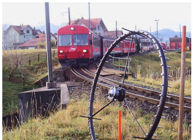
Fig. 8 Appenzeller Train passing by at measurement set up of the Acoustic Camera
