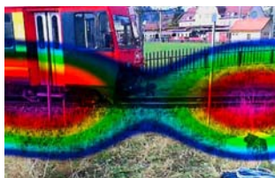
Fig. 9 Acoustic Photo 2D of an Appenzeller Bahn during Pass-by
