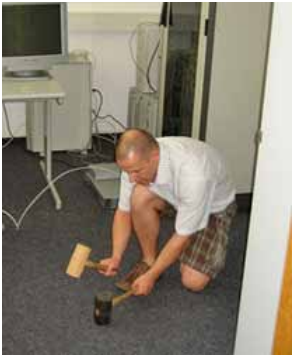
Fig. 6 Knocking with two different hammers from the office room above
