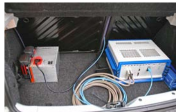
Fig. 4 Set-up of the data recorder and mobile power supply in the trunk
