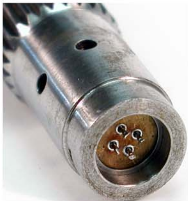
SEALED TERMINIALS AT END OF TRANSMISSION INPUT SHAFT - CONNECTED TO STRAIN GAGE TORQUE BRIDGE
