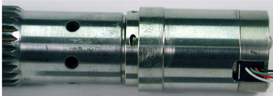
SEALED TERMINIALS AT END OF TRANSMISSION INPUT SHAFT - CONNECTED TO STRAIN GAGE TORQUE BRIDGE
